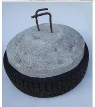
Hence, 400 kg per tire, makes 7 kN per running meter if the tires are placed in the foundation ditch one after the other. This represents the proportional weight of a brick/hollow block wall, including a concrete foundation beam and a roof structure with corrugated sheets. This is by far the most typical construction mode in poor urban areas.
