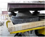
We configured four tires, one in each corner of the  $2.5 \times 2.5 \text{m}$  shake table and confined them with timber frames. On each tire a precast Elephant Foot was mounted. On top was placed a steel plate of the same dimension as the table. The load was increased from 800 kg (by the top plate itself) up to totally 1600 kg. This shake table is operating only in the x-axis. However, the horizontal forces are the most devastating in an earth quake and the most relevant to measure.
