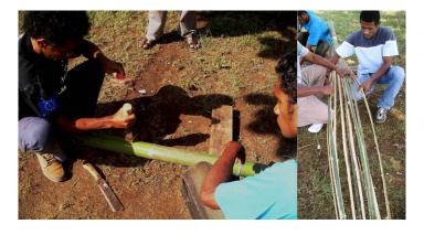
Then the entire pole is compressed from both ends and a spool shaped basket is automatically created. The noses at both ends should be reinforced with some 3 mm steel wire against splitting.
